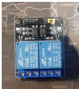
**Gambar 5. Relay 5V 2channel**
