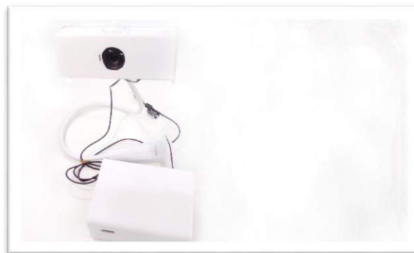
Gambar 12. Purwarupa Smart Baby Monitor
